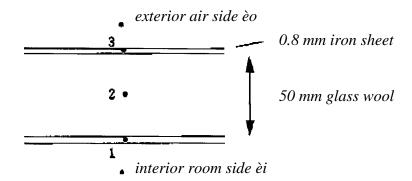
Glass wool physical property values: thermal conductivity  $\ddot{e} = 0.0377 \text{ kcal/(m}^2 \text{ x h x °C)}$  specific heat c = 0.2 kcal/(kg x °C) density  $\tilde{n} = 20 \text{ kg/m}^3$  volumetric specific heat  $= 821 \text{ kcal/(m}^3 \text{ x °C)}$
