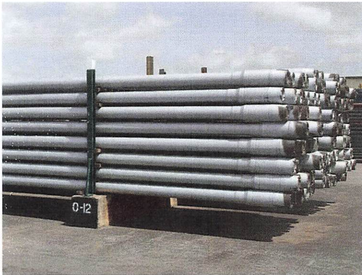
Coated 7-5/8" MaXit807 Completion Landing String
