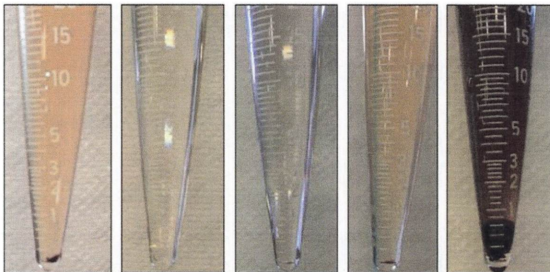
Figure 3—Four coating samples tested on pipe samples immersed in 14.2 ppg \text{CaBr}_2 fluid for 12 days against uncoated pipe sample on the right.
