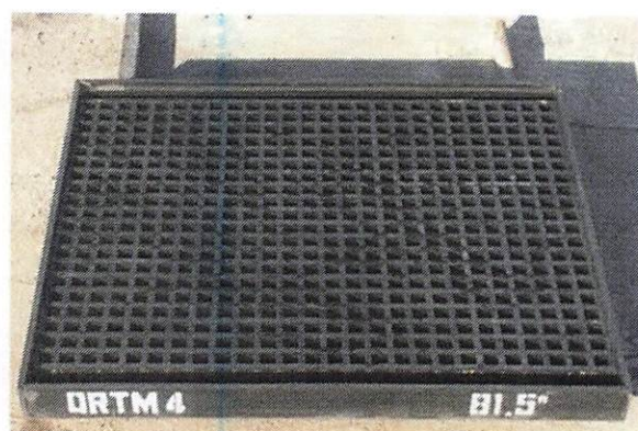
Figure 2—High-pressure pipe washing wand to rinse salt-based fluids from tubulars with optimum jet design and flowrate, and racking mats to facilitate drainage of completion fluids away from connections in order to mitigate corrosion and pitting.
