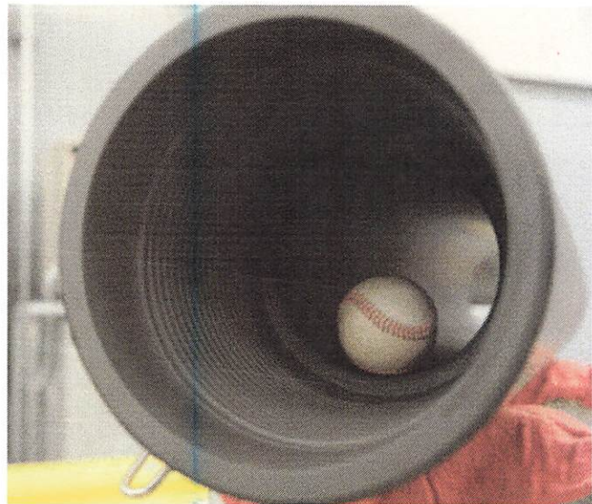
Grant Prideco's MaXit connection has a large 6 1/4-in. ID. The connection was delivered in 2016, in conjunction with a 7 5/8-in. intervention and completion landing string. The size requirement for the connection came about because the operator wanted to run a larger crown plug through it. Other technical requirements were for the connection to be gas-tight and to have a pressure rating of 20,000 psi.
